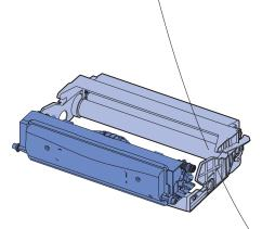
6 Install the toner cartridge assembly into the printer by aligning the green arrows on the guides of the toner cartridge assembly with the green arrows on the tracks in the printer and pushing the toner cartridge assembly in as far as it will go.
